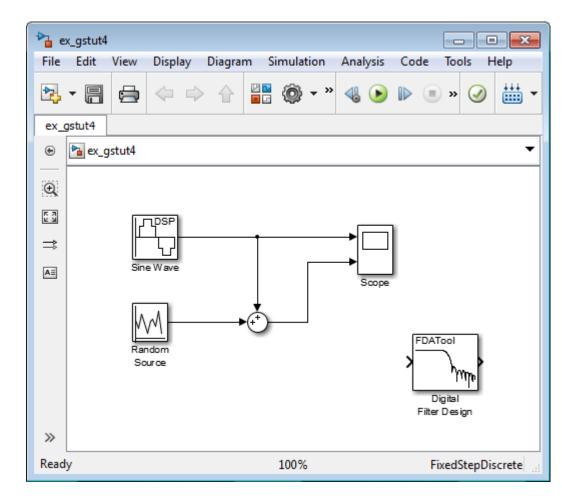
**2** Incorporate the Digital Filter Design block into your block diagram by placing it between the Random Source block and the Sum block.
